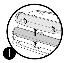
Shut down your computer, then disconnect the power adapter and phone cord. Turn the computer over and remove the battery.
