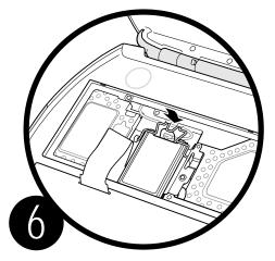
Press the wire bracket down to secure the card, then replace the keyboard and battery.
