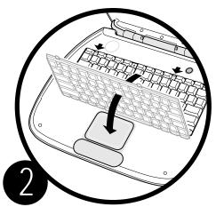
Release the keyboard by sliding the two plastic tabs away from the display. Then lift the keyboard, flip it over, and lay it on the palm rests.
