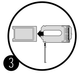
Remove the metal clip and pull the AirPort Card from the iMac AirPort Card adapter.
