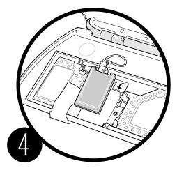
Flip up the wire bracket and connect the end of the antenna to the AirPort Card. Make sure the antenna is securely connected to the card.
