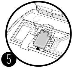
Slide the AirPort Card (with the AirPort ID number facing up) between the guides, under the wire bracket, and into the slot under the top edge of the trackpad.
