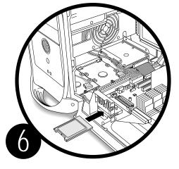
Insert the AirPort Card through the opening in the PCI card guide, and into the connector on the main logic board.
