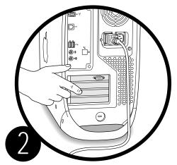
Touch the metal PCI access covers on the back of the computer to discharge static electricity.
