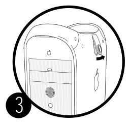
Unplug the power cord. Then lift the latch on the side of the computer.
