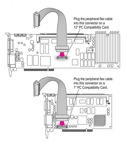
9 Insert the PC Compatibility Card into the second slot.
