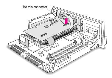
14 Push the peripheral flex cable down.
