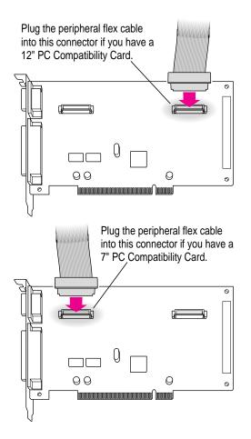
**10** Connect the peripheral flex cable to the PC Serial and Parallel Card.
