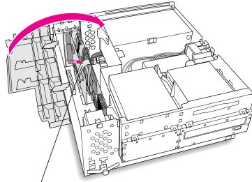
**15** Push the peripheral flex cable gently so that it bends towards the PC Compatibility Card.
