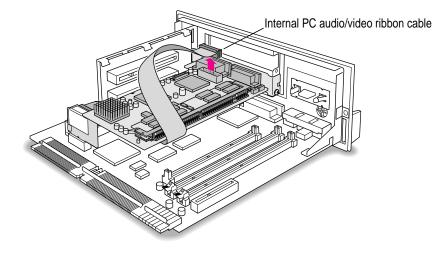
8 Disconnect the Internal PC audio/video ribbon cable from the PC Compatibility Card.
