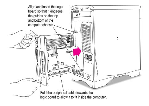
17 Align and insert the logic board part way into the computer.
