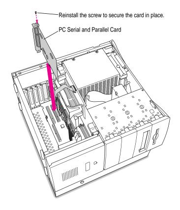
13 Reinsert the screw to secure the card in place.
