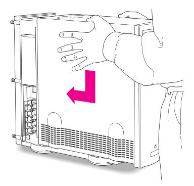
**19** Tighten the screws on the back panel and reconnect the power cord and other cables.
