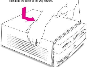
Set the cover down so there's about a quarter of an inch gap here. Then slide the cover all the way forward.
