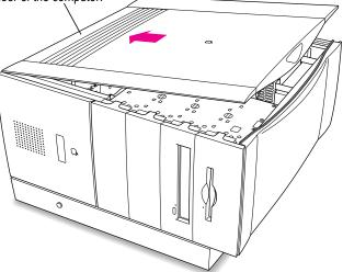
Press down on the top edge of the cover panel until it snaps firmly into place.
