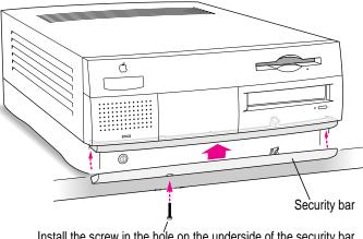
Install the screw in the hole on the underside of the security bar.
