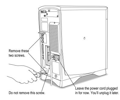
3 Touch the recessed metal parts in the back panel to discharge static electricity from your body.
