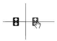
If your AppleVision monitor supports it, there are additional handles near the top and bottom of the monitor. Adjust the top convergence first, then the bottom. You may need to readjust the center convergence after moving the top or bottom.
