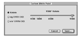
To set the white point using CIE xy or CIE u'v' color spaces, click the appropriate button; then adjust the white point by moving the crosshairs or typing values in the text boxes.
