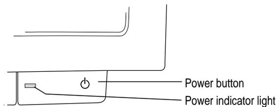
The power indicator light goes on. If the power indicator light does not come on, press the power switch again. If this doesn't work, make sure you've connected the monitor to your computer properly (see "Connecting the Monitor to Your Computer," earlier in this chapter). Also, make sure your computer is turned on.
