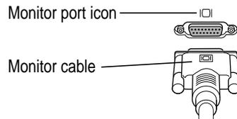
If you installed a video card in your computer, connect the monitor cable to the video card's port. For more information about installing video cards, see the manual that came with your computer or video card.
