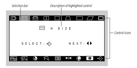
**Note:** The On-Screen Display disappears after a number of seconds if you haven't turned the Select/Adjust knob or pressed the Enter button. (You can change the number of seconds by accessing the OSD control; see the sections that follow for more information.)
