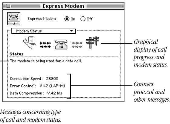
The Apple Serial Modem status display appears in the Status section of the control panel.
