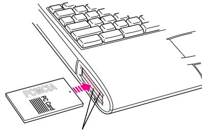
A Type I or Type II PC Card can be inserted in either the upper or lower slot.
