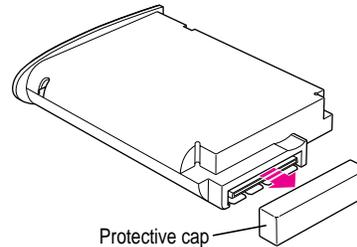
Be sure to keep the cap so that you can place it back on the module when you are not using it.
