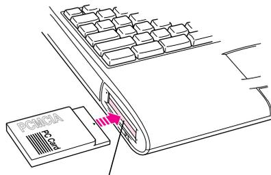
A Type III PC Card must be inserted in the lower slot.
