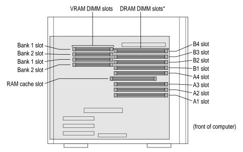
\*When installing DRAM, for best performance, fill slots A1 and B1, then A2 and B2, then A3 and B3, and so forth.
