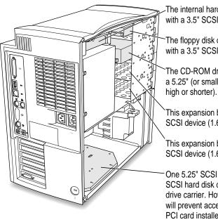
The internal hard disk drive can be replaced with a 3.5" SCSI hard disk drive (1" high).
