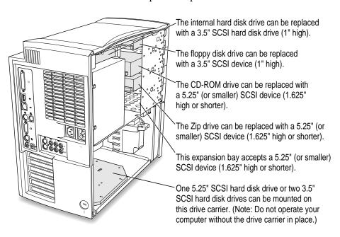
The internal SCSI chain supports "Fast" SCSI-2, which can transfer data at up to 10 MB per second (twice the rate of the external standard SCSI-2 chain). If you obtain a SCSI device that supports "Fast" SCSI-2, you should receive faster performance if it is connected to the internal SCSI chain.
