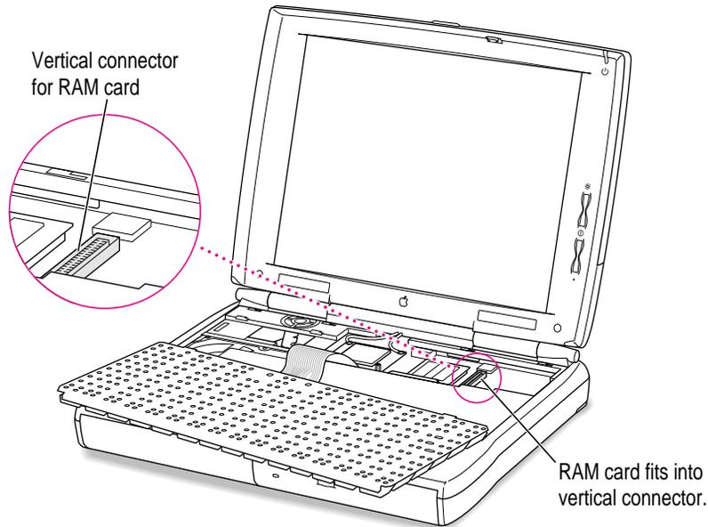
The area around the RAM card's vertical connector may be partially obscured if your computer has a card installed in the expansion card slot (not used for a RAM card).
