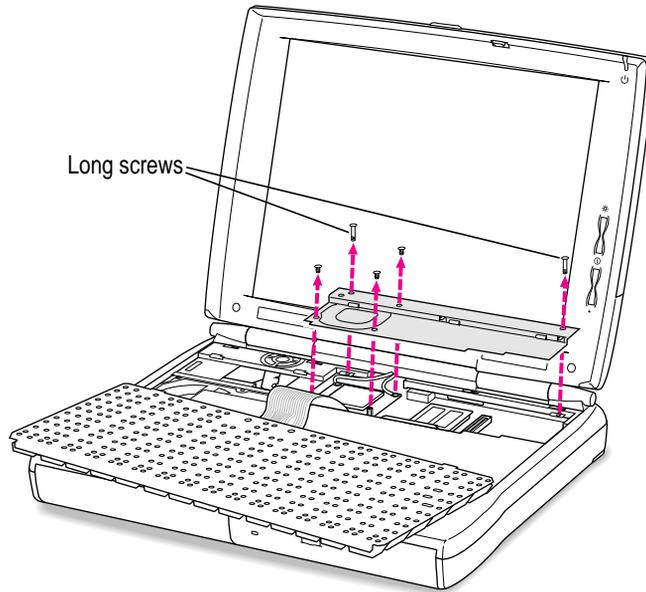
**7** Locate the vertical connector for the RAM card near the right side of the computer.
