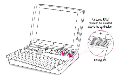
10 Lower the left side of the card so that its connector is aligned with the vertical connector in the computer and gently push the card down until it is seated.
