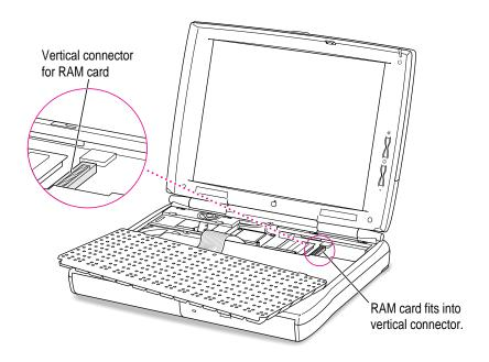
The area around the RAM card's vertical connector may be partially obscured if your computer has a card installed in the expansion card slot (not used for a RAM card). 8 Carefully remove the RAM card from its packaging and position it above the area for installation in the computer.
