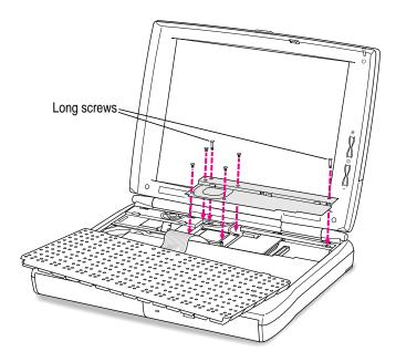
**13** Replace the keyboard by folding it backward and lowering the top edge into place.
