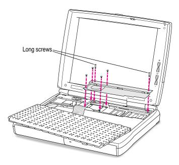
12 Replace the keyboard by folding it backward and lowering the top edge into place.
