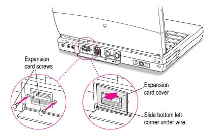
Use a small Phillips screwdriver to tighten the screws.
