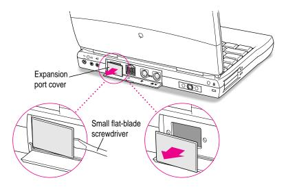
Be sure to save the cover so that you can replace it should you remove the expansion slot card later.
