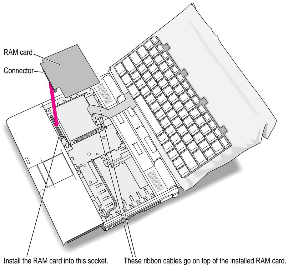
**15 Lay the card flat, then gently press the card into the socket.**
