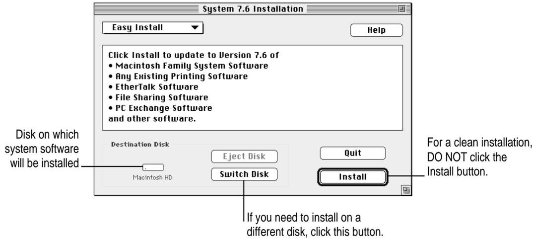
**11 Make sure that the hard disk named in the Destination Disk box is the one on which you want to install system software.**
