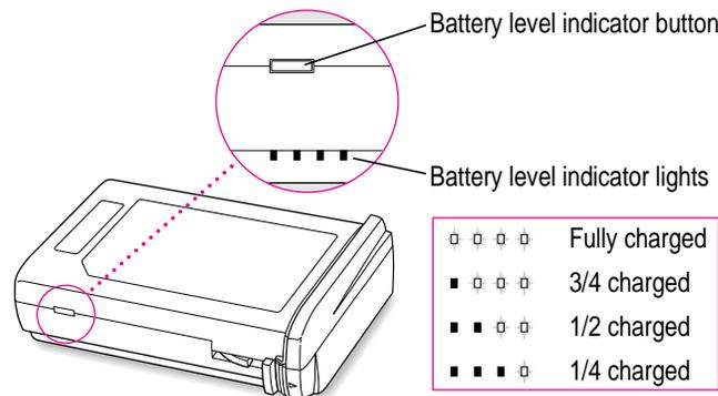
**IMPORTANT** If the battery lights are blinking, there’s a problem with the battery. See an Apple-authorized service provider for assistance.
