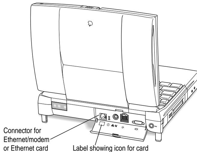
If your PowerBook has an expansion card installed, the cable or cables you need to use the card are also supplied with the computer.
