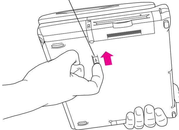
**4** Hold the module by the gripping surface and pull it out of the computer.
