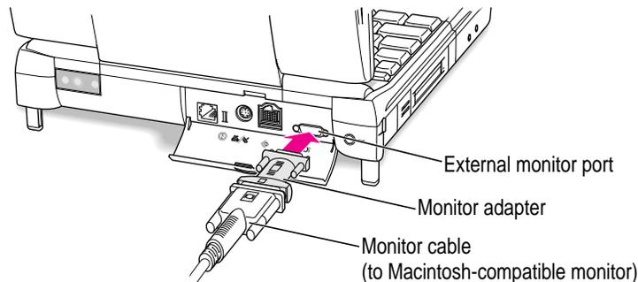
If you are connecting a VGA or SVGA monitor, do not use the adapter. Connect the monitor cable directly to the external monitor port on the PowerBook.
