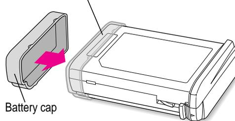
The battery contacts should not be exposed when the battery is out of the computer.
