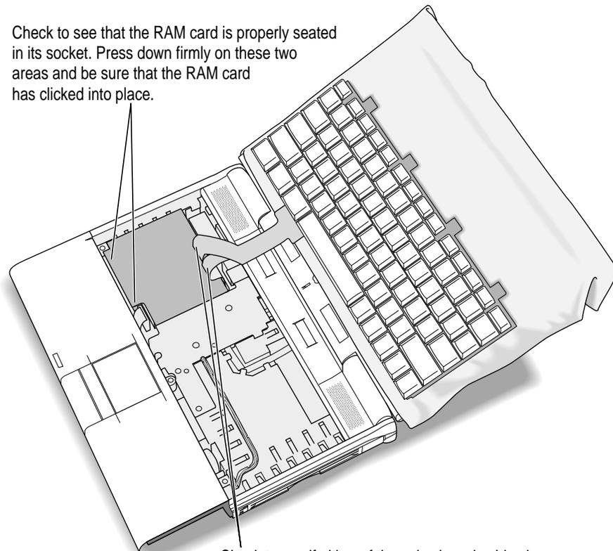
Check to see if either of these keyboard cables has been pulled out of its socket on the logic board.
