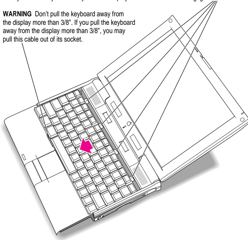
This action should release the top edge of the keyboard from its enclosure, allowing you to grasp and free the entire keyboard.
