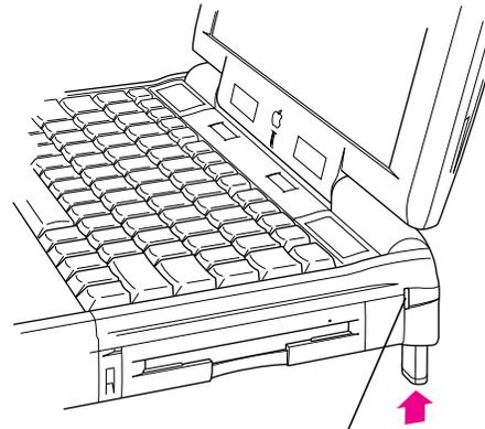
To raise the foot, press the release button while pushing up on the foot until it clicks into place.
