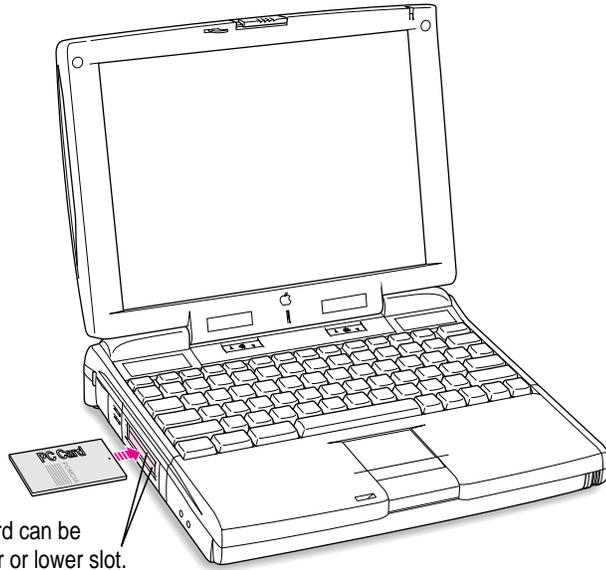
A Type I or Type II PC Card can be inserted in either the upper or lower slot.
