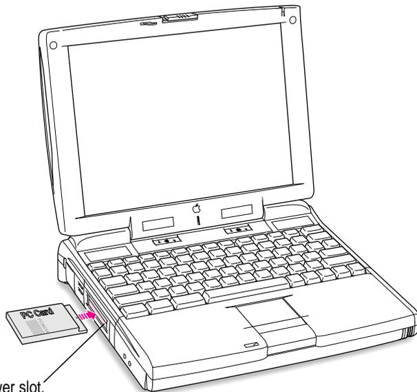
A Type III PC Card must be inserted in the lower slot.
