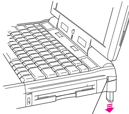
To lower the foot, press the release button. The foot extends automatically.
