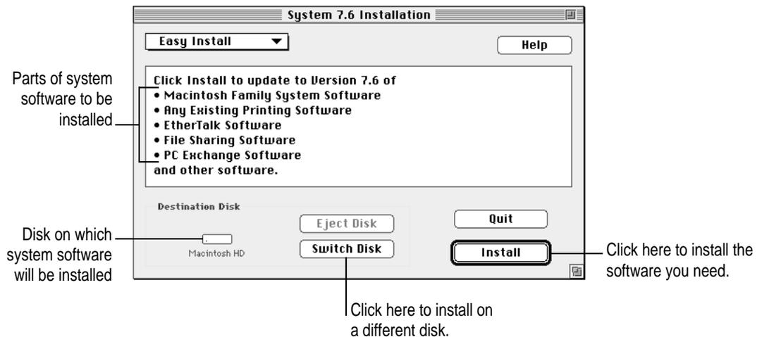
**11 Make sure that the hard disk named in the box is the one on which you want to install system software.**
