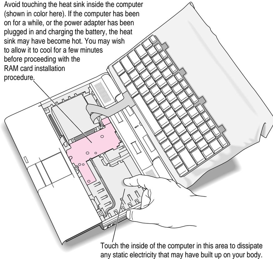
Touch the inside of the computer in this area to dissipate any static electricity that may have built up on your body.
