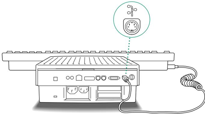
**5. Now connect any other equipment you have, such as an external hard disk drive or printer.**
