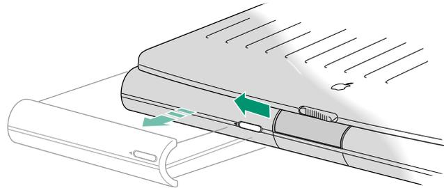
4. **Carefully pull the battery out of its compartment.**
