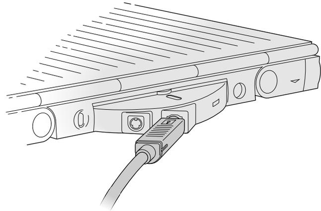
4. **If you are using an external keyboard or a mouse, connect its cable to the Apple Desktop Bus (ADB) port on the adapter. The port is marked with this icon:**
