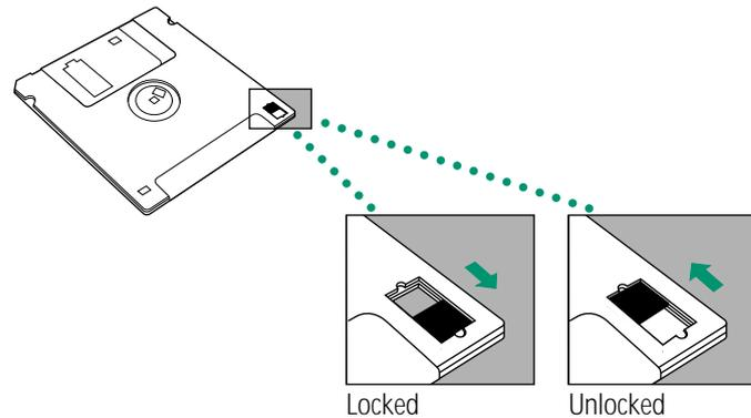
To unlock the disk, slide the tab back so that it covers the square hole.
