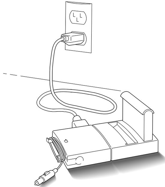
3. **Place the battery in the recharger as shown.**
