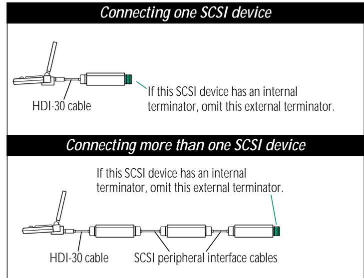
△ **Important:** The total length of a SCSI chain should not exceed 6 meters (20 feet). Apple SCSI cables are designed to meet this restriction. If you are using SCSI cables from another vendor, check the length of the chain. △
