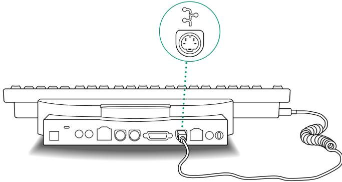
5. If you are using an external floppy disk drive, connect its cable to the floppy disk drive port (marked with the icon
