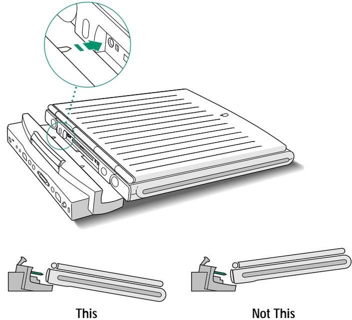
4. **Push down on the latch at the top of the minidock to secure the connection.**
