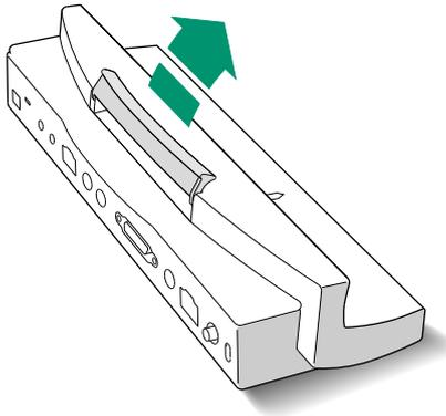
3. **Slide the posts on the minidock into the corresponding holes on the back of the PowerBook, and then gently push the two devices together.**
