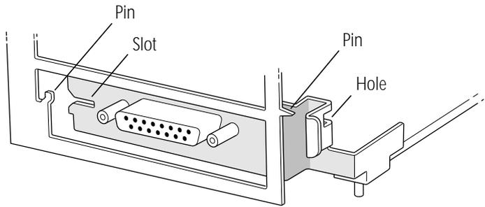
**13. Press together the connectors on the card and the slot.**
