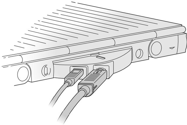
If you plan to use the computer's battery as your power source, the battery charge will last longer if you use ADB devices designed for portable computers. These devices are marked with this low-power icon:
