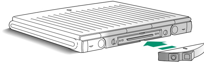
**3. Connect the floppy disk drive's cable to the floppy disk drive port on the adapter. The port is marked with this icon:
