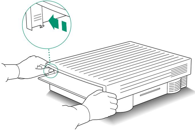
2. When the latches release, tilt the cover upward slightly (to about a 30° angle) and then lift the angled cover straight up to remove it.
