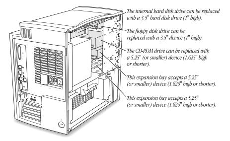
An Apple-authorized dealer or service provider can replace existing internal storage devices with others, along with any necessary data cables or brackets to secure each device inside the computer.
