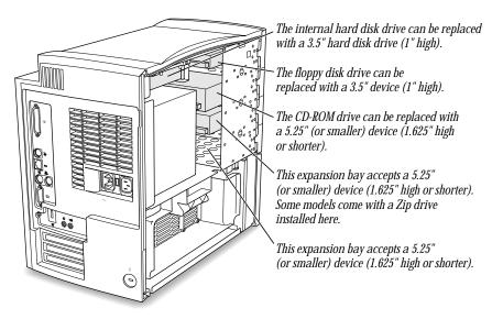
An Apple-authorized dealer or service provider can replace existing internal storage devices with other ones, along with any necessary data cables or brackets to secure each device inside the computer.
