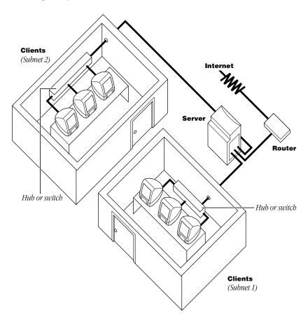
In this configuration, the server acts as a router to one or more NetBoot client subnets. If this is your configuration, select Gateway in the IP Routing Configuration panel of the NetBoot Server Setup Assistant. You do not need to provide a router address.
