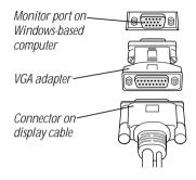
2 Tighten the thumbscrews on the connector.
