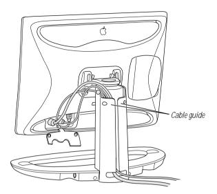
The ADB cable has a plastic cable capture in the middle of the cable. This capture allows slack in the ADB cable so the cable won't get damaged when you adjust the display.
