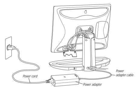
2 Plug one end of the power cord into the power adapter and the other end into a three-hole grounded outlet or power strip.
