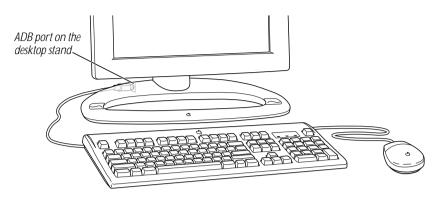
When connecting ADB cables, make sure you align the symbol on the connector with the same symbol on the port. If you force a connector the wrong way, you will damage it. Make sure the ADB connector is attached firmly.
