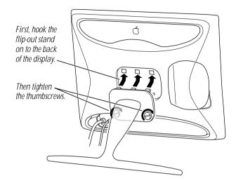
**3** Place the bottom part of the cover against the display and screw in the two plastic thumbscrews.
