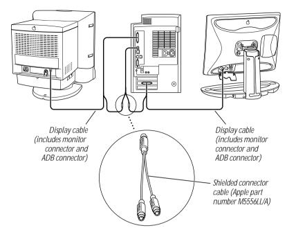
**Important** Make sure you use an Apple shielded connector cable. Most third-party ADB splitter cables are not shielded and will not work properly with your display. You may experience more radio interference with an unshielded connector cable.
