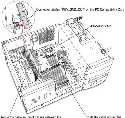
Route the cable so that it passes between the processor card and the PC Compatibility Card.
