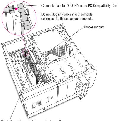
Route the cable so that it passes between the processor card and the PC Compatibility Card.
