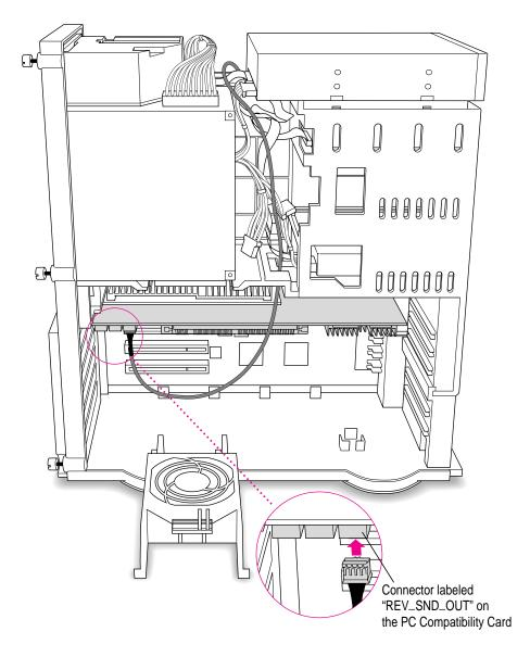
15 Plug the other SCSI audio cable into the back of the CD-ROM drive.
