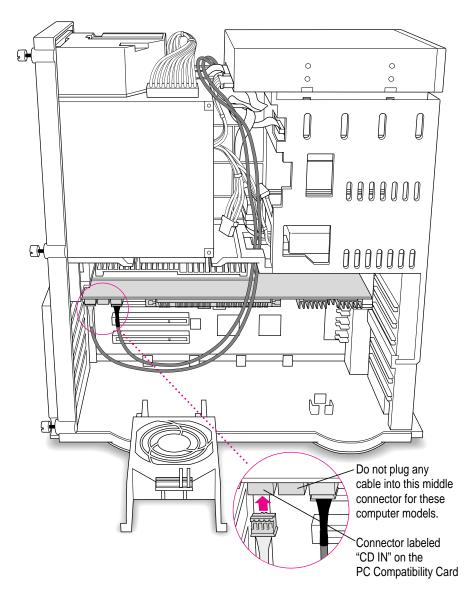
Installing the Card in a Power Macintosh 8500 or 9500
