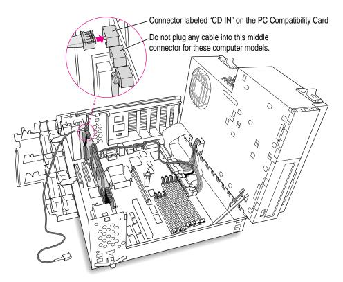
22 Route the second cable over the top of the card, around the back of the logic board, and through the hole in the computer's chassis.
