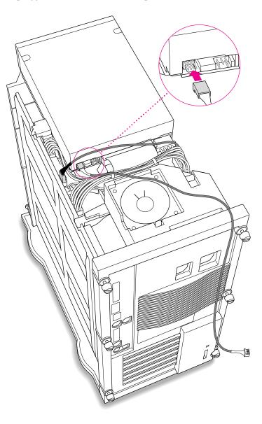
Installing the Card in a Power Macintosh 8500 or 9500
