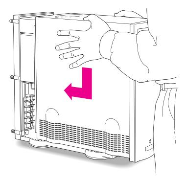
23 Tighten the screws on the back panel and reconnect the power cord and other equipment cables.
