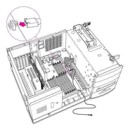
17 Plug the other end of the SCSI audio cable into the connector labeled "REV\_SND\_OUT" (Reversed Sound Out) on the PC Compatibility Card.
