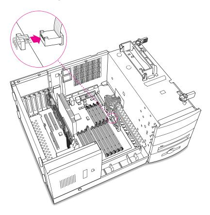
16 Plug one of the two identical SCSI audio cables (with the plug shown below) into the connector on the logic board.
