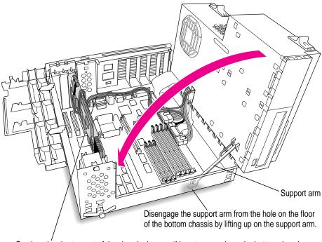
Gently swing the top part of the chassis down until it rests securely on the bottom chassis. Be sure that you don't pinch any of the cables between the top and bottom parts of the chassis.
