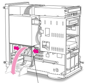
To lower the retainer, squeeze the sides to unlatch it.
