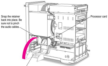
This guide on the retainer engages the processor card in the computer.
