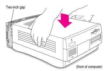
**31** Lower the cover onto the case, leaving a two-inch gap, and then push the cover back.
