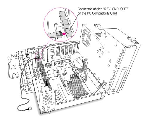
20 Route the cable over the top of the card and around the back of the Macintosh logic board. Then plug the cable into the audio connector on the logic board.
