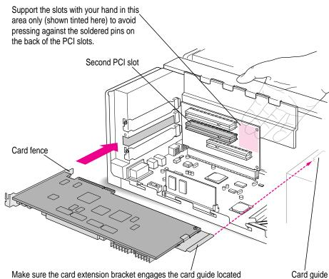
Make sure the card extension bracket engages the card guide located on the speaker housing inside the front of the computer.
