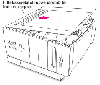
Press down on the top edge of the cover panel until it snaps firmly into place.
