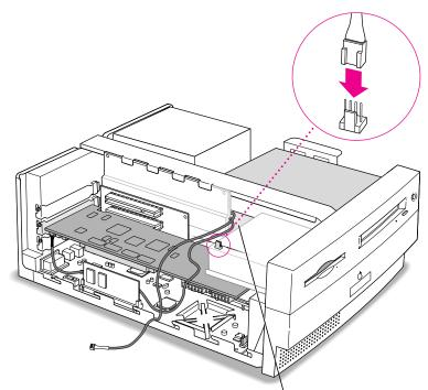
Route the cable so that it passes under the support bar and through the opening.
