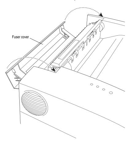
Align the V-shaped blocks under the duplex printing unit with the holes located on the fuser cover and gently place the duplex printing unit on top of the printer.
