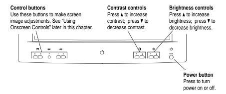
The contrast and brightness controls have an onscreen indicator that appears when you press the contrast and brightness control buttons on the front of your monitor. When you make an adjustment, the indicator bar moves to show the current setting. When you've finished making adjustments, the indicator disappears automatically.
