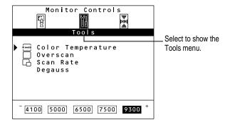
Use the Tools menu to set color temperature, turn overscan on and off, display the scan rate of your monitor, and manually degauss.
