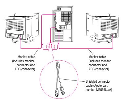
**IMPORTANT** Make sure you use an Apple *shielded* connector cable. Most third-party ADB splitter cables are not shielded and will not work properly with your ColorSync monitor. (You may experience more radio interference with an unshielded connector cable.)
