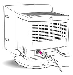
Plug the other end of the power cord into a grounded outlet or power strip.
