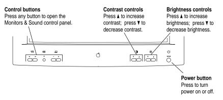
The Contrast and Brightness controls have an onscreen indicator that appears when you press a button on the front of your monitor. For example, pressing a Brightness control displays the Brightness indicator.
