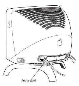
2 Plug the other end of the power jumper cord (which plugs into the power socket on other equipment) into the power socket on the back of your computer.
