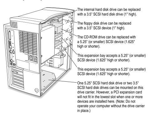
The internal SCSI chain supports "Fast" SCSI, which is capable of transferring data at up to 10 MB per second (twice the rate of the external standard SCSI chain). If you obtain a SCSI device that supports "Fast" SCSI, you should receive faster performance if it is connected to the internal SCSI chain.
