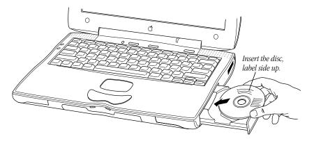
**Note:** CD-ROM and DVD-ROM drives have small locks on the drive spindle that securely hold the disc in place. When inserting a disc over these locks, you may need to apply additional pressure. Place the hole in the center of the disc directly over the drive spindle and press down until you feel the disc lock into place.
