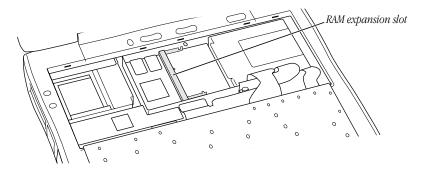
Gently touch the metal surface on the right side of the inside of the computer to discharge any static electricity built up on your body.
