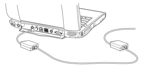
4 If you are using a LocalTalk adapter with RJ-11 (telephone) connectors, connect a terminator to the unused RJ-11 connector on the LocalTalk adapter. A LocalTalk adapter with DIN-8 connectors doesn't require an external terminator. (For more information on terminators, see the instructions that came with the Apple LocalTalk RJ-11 Connector Kit.)
