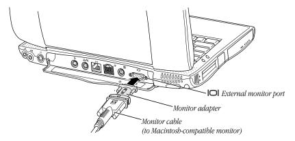
If you are connecting a VGA or SVGA monitor, do not use the adapter. Connect the monitor cable directly to the external monitor port on the PowerBook.
