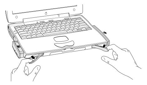
**6** Remove the modules or batteries from both the expansion bays.
