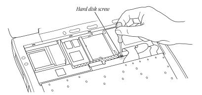
**5** Gently pull up on the small metal tab (located on the left side of the hard disk) to disengage the hard disk from the logic board.
