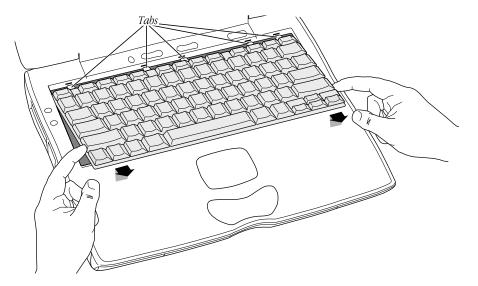
10 Flip the keyboard over and lay it on the palm rests and trackpad.
