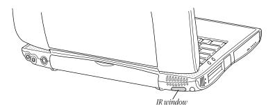
With IR communications, you can exchange files with another PowerBook or with a desktop Macintosh using an external IR module. You can also use IR to make a wireless connection to a network by means of a specialized local area network (LAN) access device that is compatible with the Infrared Data Association (IrDA) Standard specifications.
