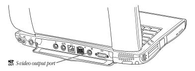
Warning The S-video output port (labeled with the ♣ icon) looks similar to the ADB port (labeled with the ♣ icon) and the printer/modem port (labeled with the ♣ icon). Only plug your S-video device into the S-video output port. Plugging a video device into the wrong port could damage your equipment.
