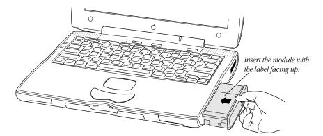
**Note:** The right expansion bay can accept the wide 5.25-inch CD-ROM or DVD-ROM drive module or the narrower floppy disk drive module or PowerBook battery. When a narrower device is in the expansion bay, a small flap covers the empty part of the bay. When the wider CD-ROM or DVD-ROM drive module is inserted, the flap folds into the bay.
