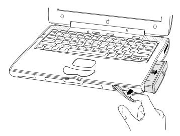
When the lever is completely extended, the module will be partially out of the expansion bay.
