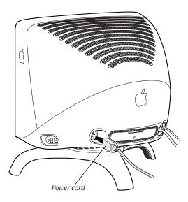
2 Plug the other end of the power jumper cord (which plugs into the power socket on other equipment) into the power socket on the back of your computer.
